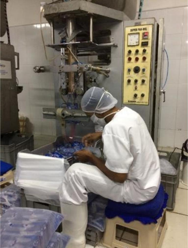
A photograph showing a worker in a white uniform and cap operating a machine labeled 'SUPER PAK-ME'. The worker is sitting on a blue cushioned stool and is leaning forward, working with a tray of blue plastic bags. The machine is a complex industrial device with various components and a control panel with several buttons and a gauge. |
