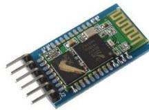
**Figura 23**, modulo bluetooth hc-05, Recuperado de [http://botscience.net/store/image/cache/data/products/MODCOM/TEL0001/Bluetooth\\_Module\\_bb-500x500.jpg](http://botscience.net/store/image/cache/data/products/MODCOM/TEL0001/Bluetooth_Module_bb-500x500.jpg)
